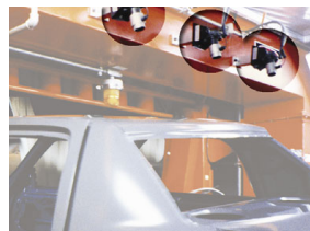
(3) Gen4 Ion Air Cannons blow contaminants from car bodies prior to painting.
