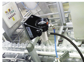
The Model 8292 Gen4 Ion Air Cannon System eliminates the static and dust prior to filling the bottles.
